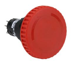
Fuji Electric emergency stop pushbutton, IP65, 16mm, push to lock, pull or turn to reset, (4) N.C. contact(s), plastic base, plastic bezel, black, Operator: red, mushroom, 40mm, mushroom, plastic.
