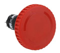
Fuji Electric emergency stop pushbutton, IP65, 16mm, push to lock, pull or turn to reset, (2) N.C. contact(s), plastic base, plastic bezel, black, Operator: red, mushroom, 40mm, mushroom, plastic.
