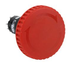
Fuji Electric emergency stop pushbutton, IP65, 16mm, push to lock, pull or turn to reset, LED illuminated, (1) N.O./(3) N.C. contact(s), plastic base, plastic bezel, black, Operator: red, mushroom, 40mm, mushroom, plastic, 24 VAC/VDC, full voltage.
