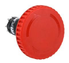
Fuji Electric emergency stop pushbutton, IP65, 16mm, push to lock, pull or turn to reset, LED illuminated, (1) N.O./(2) N.C. contact(s), plastic base, plastic bezel, black, Operator: red, mushroom, 40mm, mushroom, plastic, 24 VAC/VDC, full voltage.
