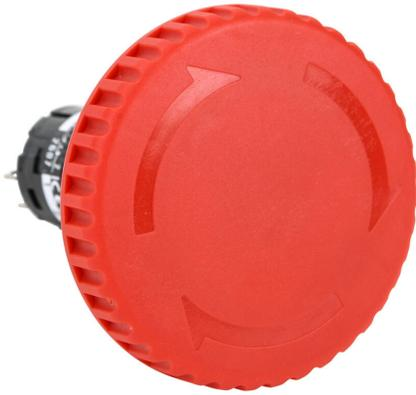
Fuji Electric emergency stop pushbutton, IP65, 16mm, push to lock, pull or turn to reset, LED illuminated, (2) N.C. contact(s), plastic base, plastic bezel, black, Operator: red, mushroom, 40mm, mushroom, plastic, 24 VAC/VDC, full voltage.
