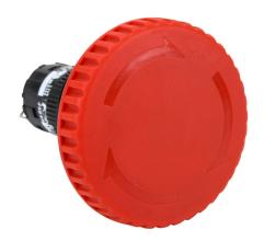
Fuji Electric emergency stop pushbutton, IP65, 16mm, push to lock, pull or turn to reset, LED illuminated, (1) N.C. contact(s), plastic base, plastic bezel, black, Operator: red, mushroom, 40mm, mushroom, plastic, 24 VAC/VDC, full voltage.
