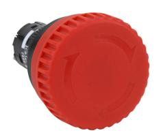
Fuji Electric emergency stop pushbutton, IP65, 16mm, push to lock, pull or turn to reset, (2) N.C. contact(s), plastic base, plastic bezel, black, Operator: red, mushroom, 32mm, mushroom, plastic.
