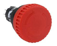
Fuji Electric emergency stop pushbutton, IP65, 16mm, push to lock, pull or turn to reset, LED illuminated, (1) N.O./(3) N.C. contact(s), plastic base, plastic bezel, black, Operator: red, mushroom, 32mm, mushroom, plastic, 24 VAC/VDC, full voltage.
