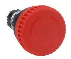
Fuji Electric emergency stop pushbutton, IP65, 16mm, push to lock, pull or turn to reset, LED illuminated, (1) N.O./(2) N.C. contact(s), plastic base, plastic bezel, black, Operator: red, mushroom, 32mm, mushroom, plastic, 24 VAC/VDC, full voltage.
