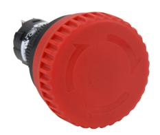
Fuji Electric emergency stop pushbutton, IP65, 16mm, push to lock, pull or turn to reset, LED illuminated, (1) N.O./(1) N.C. contact(s), plastic base, plastic bezel, black, Operator: red, mushroom, 32mm, mushroom, plastic, 24 VAC/VDC, full voltage.
