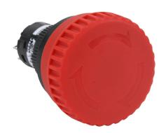
Fuji Electric emergency stop pushbutton, IP65, 16mm, push to lock, pull or turn to reset, LED illuminated, (2) N.C. contact(s), plastic base, plastic bezel, black, Operator: red, mushroom, 32mm, mushroom, plastic, 24 VAC/VDC, full voltage.
