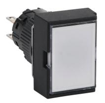
Fuji Electric pushbutton, IP65, 16mm, push ON - push OFF, DPDT contact(s), plastic base, plastic bezel, black, guarded, Operator: white, flush, 24mm, rectangular, plastic.
