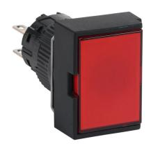
Fuji Electric pushbutton, IP65, 16mm, push ON - push OFF, DPDT contact(s), plastic base, plastic bezel, black, guarded, Operator: red, flush, 24mm, rectangular, plastic.
