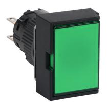
Fuji Electric pushbutton, IP65, 16mm, push ON - push OFF, DPDT contact(s), plastic base, plastic bezel, black, guarded, Operator: green, flush, 24mm, rectangular, plastic.
