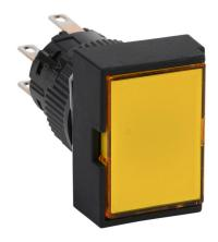
Fuji Electric pushbutton, IP65, 16mm, push ON - push OFF, LED illuminated, DPDT contact(s), plastic base, plastic bezel, black, guarded, Operator: yellow, flush, 24mm, rectangular, plastic, 24 VAC/VDC, full voltage.
