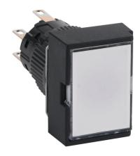
Fuji Electric pushbutton, IP65, 16mm, push ON - push OFF, LED illuminated, DPDT contact(s), plastic base, plastic bezel, black, guarded, Operator: white, flush, 24mm, rectangular, plastic, 24 VAC/VDC, full voltage.
