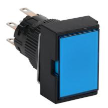
Fuji Electric pushbutton, IP65, 16mm, push ON - push OFF, LED illuminated, DPDT contact(s), plastic base, plastic bezel, black, guarded, Operator: blue, flush, 24mm, rectangular, plastic, 24 VAC/VDC, full voltage.
