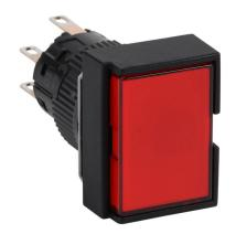
Fuji Electric pushbutton, IP65, 16mm, push ON - push OFF, LED illuminated, DPDT contact(s), plastic base, plastic bezel, black, guarded, Operator: red, flush, 24mm, rectangular, plastic, 24 VAC/VDC, full voltage.
