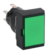
Fuji Electric pushbutton, IP65, 16mm, push ON - push OFF, LED illuminated, DPDT contact(s), plastic base, plastic bezel, black, guarded, Operator: green, flush, 24mm, rectangular, plastic, 24 VAC/VDC, full voltage.
