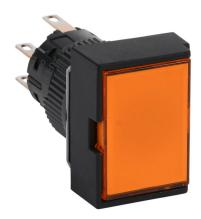
Fuji Electric pushbutton, IP65, 16mm, push ON - push OFF, LED illuminated, DPDT contact(s), plastic base, plastic bezel, black, guarded, Operator: orange, flush, 24mm, rectangular, plastic, 24 VAC/VDC, full voltage.
