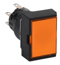
Fuji Electric pushbutton, IP65, 16mm, push ON - push OFF, LED illuminated, DPDT contact(s), plastic base, plastic bezel, black, guarded, Operator: orange, flush, 24mm, rectangular, plastic, 24 VAC/VDC, full voltage.
