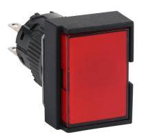
Fuji Electric pushbutton, IP65, 16mm, momentary, DPDT contact(s), plastic base, plastic bezel, black, guarded, Operator: red, flush, 24mm, rectangular, plastic.
