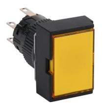
Fuji Electric pushbutton, IP65, 16mm, momentary, LED illuminated, DPDT contact(s), plastic base, plastic bezel, black, guarded, Operator: yellow, flush, 24mm, rectangular, plastic, 24 VAC/VDC, full voltage.
