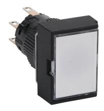
Fuji Electric pushbutton, IP65, 16mm, momentary, LED illuminated, DPDT contact(s), plastic base, plastic bezel, black, guarded, Operator: white, flush, 24mm, rectangular, plastic, 24 VAC/VDC, full voltage.
