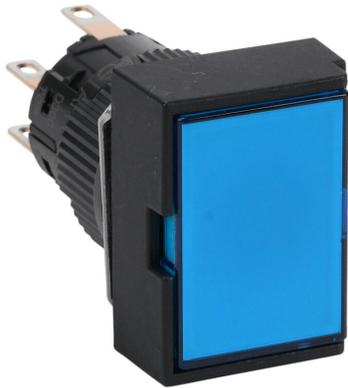
Fuji Electric pushbutton, IP65, 16mm, momentary, LED illuminated, DPDT contact(s), plastic base, plastic bezel, black, guarded, Operator: blue, flush, 24mm, rectangular, plastic, 24 VAC/VDC, full voltage.
