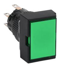
Fuji Electric pushbutton, IP65, 16mm, momentary, LED illuminated, DPDT contact(s), plastic base, plastic bezel, black, guarded, Operator: green, flush, 24mm, rectangular, plastic, 24 VAC/VDC, full voltage.
