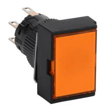
Fuji Electric pushbutton, IP65, 16mm, momentary, LED illuminated, DPDT contact(s), plastic base, plastic bezel, black, guarded, Operator: orange, flush, 24mm, rectangular, plastic, 24 VAC/VDC, full voltage.
