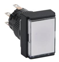
Fuji Electric pushbutton, IP65, 16mm, push ON - push OFF, LED illuminated, DPDT contact(s), plastic base, plastic bezel, black, Operator: white, flush, 24mm, rectangular, plastic, 24 VAC/VDC, full voltage.
