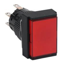
Fuji Electric pushbutton, IP65, 16mm, push ON - push OFF, LED illuminated, DPDT contact(s), plastic base, plastic bezel, black, Operator: red, flush, 24mm, rectangular, plastic, 24 VAC/VDC, full voltage.
