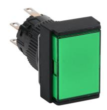
Fuji Electric pushbutton, IP65, 16mm, push ON - push OFF, LED illuminated, DPDT contact(s), plastic base, plastic bezel, black, Operator: green, flush, 24mm, rectangular, plastic, 24 VAC/VDC, full voltage.
