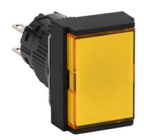
Fuji Electric pushbutton, IP65, 16mm, momentary, DPDT contact(s), plastic base, plastic bezel, black, Operator: yellow, flush, 24mm, rectangular, plastic.
