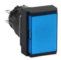
Fuji Electric pushbutton, IP65, 16mm, momentary, DPDT contact(s), plastic base, plastic bezel, black, Operator: blue, flush, 24mm, rectangular, plastic.
