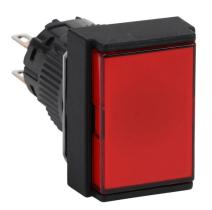
Fuji Electric pushbutton, IP65, 16mm, momentary, DPDT contact(s), plastic base, plastic bezel, black, Operator: red, flush, 24mm, rectangular, plastic.
