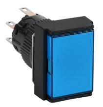
Fuji Electric pushbutton, IP65, 16mm, momentary, LED illuminated, DPDT contact(s), plastic base, plastic bezel, black, Operator: blue, flush, 24mm, rectangular, plastic, 24 VAC/VDC, full voltage.
