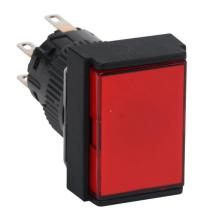
Fuji Electric pushbutton, IP65, 16mm, momentary, LED illuminated, DPDT contact(s), plastic base, plastic bezel, black, Operator: red, flush, 24mm, rectangular, plastic, 24 VAC/VDC, full voltage.
