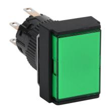
Fuji Electric pushbutton, IP65, 16mm, momentary, LED illuminated, DPDT contact(s), plastic base, plastic bezel, black, Operator: green, flush, 24mm, rectangular, plastic, 24 VAC/VDC, full voltage.
