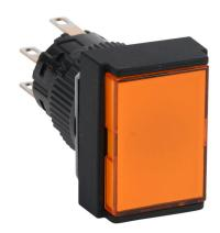
Fuji Electric pushbutton, IP65, 16mm, momentary, LED illuminated, DPDT contact(s), plastic base, plastic bezel, black, Operator: orange, flush, 24mm, rectangular, plastic, 24 VAC/VDC, full voltage.
