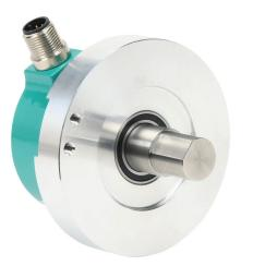
Lika Electronic AR01 series incremental (quadrature) rotary encoder, replacement, medium duty, 5-30 VDC, radial exit, universal (line driver or NPN/PNP open collector) output, 1250ppr, 15mm dual shaft, 58mm diameter body, IP65, M12 male.
