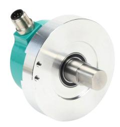
Lika Electronic AR01 series incremental (quadrature) rotary encoder, replacement, medium duty, 5-30 VDC, radial exit, universal (line driver or NPN/PNP open collector) output, 250 ppr, 15mm dual shaft, 58mm diameter body, IP65, M12 male.
