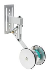
Lika Electronic AR01 series incremental (quadrature) rotary measuring wheel encoder assembly, 5-30 VDC, universal (line driver or NPN/PNP open collector) output, 1250 ppr. (1) encoder, (2) measuring wheels, (1) spring-loaded arm and (1) mounting bracket included.
