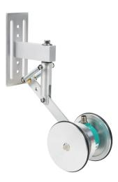
Lika Electronic AR01 series incremental (quadrature) rotary measuring wheel encoder assembly, 5-30 VDC, universal (line driver or NPN/PNP open collector) output, 250 ppr. (1) encoder, (2) measuring wheels, (1) spring-loaded arm and (1) mounting bracket included.
