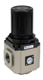
NITRA pneumatic regulator, 1in female NPT inlet(s), 1in female NPT outlet(s), 20-130 psi adjustable range. For use with Ax-68 series air prep components.
