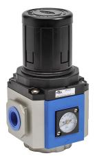
NITRA pneumatic regulator, 1/2in female NPT inlet(s), 1/2in female NPT outlet(s), 20-130 psi adjustable range. For use with Ax-44 series air prep components.
