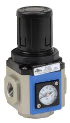
NITRA pneumatic regulator, 3/8in female NPT inlet(s), 3/8in female NPT outlet(s), 4-57 psi adjustable range. For use with Ax-33 series air prep components.
