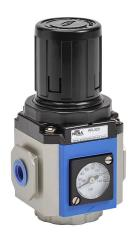
NITRA pneumatic regulator, 1/4in female NPT inlet(s), 1/4in female NPT outlet(s), 20-130 psi adjustable range. For use with Ax-32 series air prep components.
