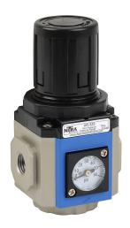
NITRA pneumatic regulator, 1/4in female NPT inlet(s), 1/4in female NPT outlet(s), 4-57 psi adjustable range. For use with Ax-32 series air prep components.
