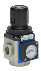
NITRA pneumatic regulator, 1/4in female NPT inlet(s), 1/4in female NPT outlet(s), 20-130 psi adjustable range. For use with Ax-22 series air prep components.
