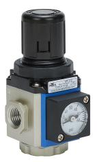
NITRA pneumatic regulator, 1/4in female NPT inlet(s), 1/4in female NPT outlet(s), 4-57 psi adjustable range. For use with Ax-22 series air prep components.
