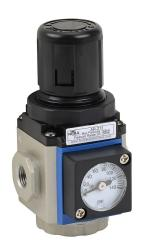
NITRA pneumatic regulator, 1/8in female NPT inlet(s), 1/8in female NPT outlet(s), 20-130 psi adjustable range. For use with Ax-21 series air prep components.
