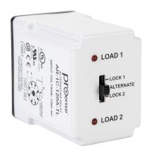
ProSense alternating relay, socket mount, finger-safe, 120 VAC coil voltage, SPDT, (1) N.O., (1) N.C., 10A contact rating, 8-pin, LED indicator(s). Relay becomes UL listed when used with 70169-D relay socket.
