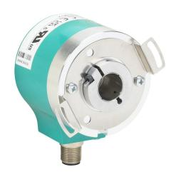
Lika Electronic AQ59 series incremental (quadrature) rotary encoder, medium duty, 5-30 VDC, radial exit, universal (line driver or NPN/PNP open collector) output, up to 14-bit (16384 ppr), multiple shafts (6mm - 15mm), 59mm diameter body, IP65, M12 male.
